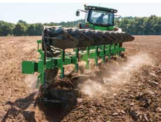
material allowing the plough to operate in adverse field conditions. The model 3910 can have 9 to 13 casings. It performs well in couple with JD 8R and 9R tractors, engine capacity 310 to 460 hp. The plough 3910 has two front bearing wheels and one rear support wheel. They guide the plough over the furrow, which makes it possible to maintain the set tilling depth. Due to its strong design, the plough can operate in all weather conditions.
