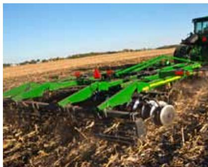
residues, loosens and breaks dense soil layers and levels out the soil surface.
