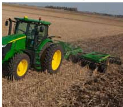
on large and small farms. The disc harrows 2623 are ideal for high load operations. By using a single point system of depth control, it is possible to precisely adjust the tilling depth. The C-shaped springs ensure operation at an equal depth all over the field, improving the harrow flexibility and protecting the discs against damage. Hydraulic longitudinal levelling makes it possible to easily control the harrow from the tractor cabin.
