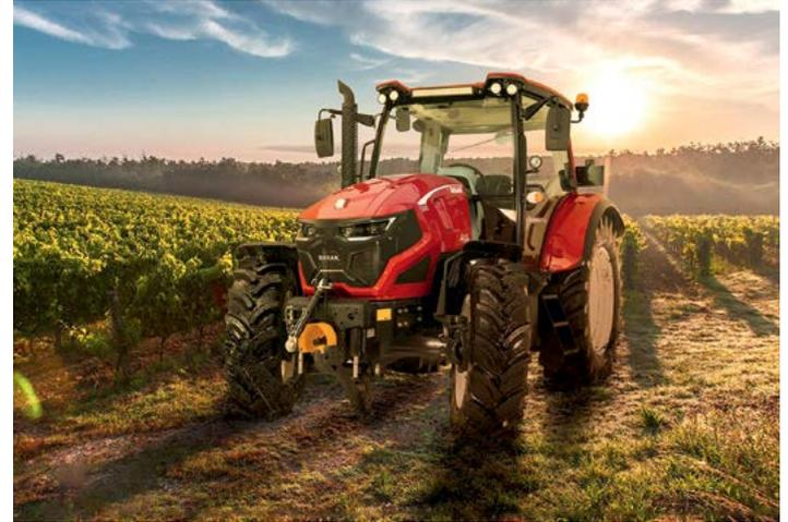
features a 116 hp 4-cylinder diesel engine with Turbo/ Intercooler from Deutz and the Common Rail fuel injection system. The unit is enhanced with the 4-speed synchronised PowerShift transmission produced by ZF with 32 forward and 32 reverse gears, electro-hydraulic gear shifting and a four-wheel drive.
