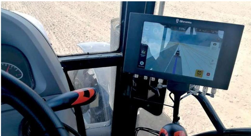
Since 2021, the Smart Farming Department of EkoNiva-Tekhnika Holding has been offering its customers the FJDynamics auto steer system, which navigates agricultural vehicles along a straight line, curves or concentric circles. Company specialists demonstrated to the clients how the equipment is used in the Russian fields.
