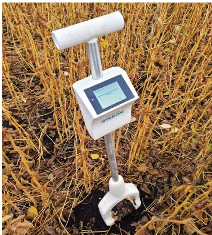
'The system has a built-in GPS-module to determine the precise coordinates of the explored area, which is key to establishing the differences in the nutrient content across the field. Besides, the lab features embedded field mapping software which provides fertiliser application guidelines. All the data is immediately uploaded to the server and promptly processed. The user has an instant access to the records via a dedicated app', continues Artyom Novikov.
