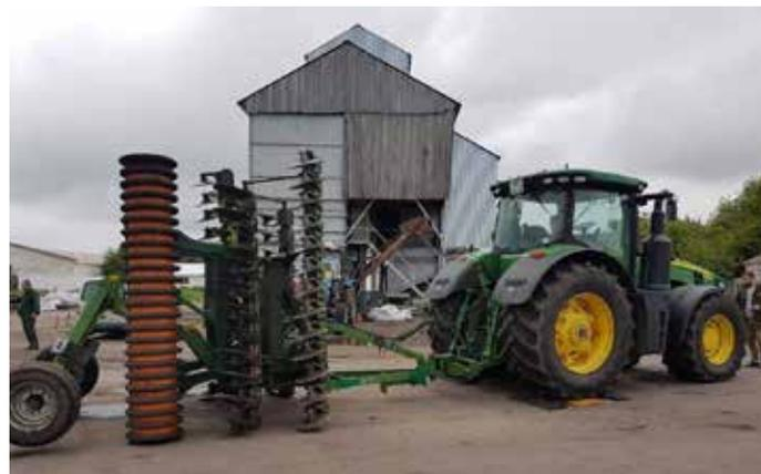
first at the front-axle side, then at the rear-axle side. We compared the load distribution between the axles depending on the equipment position. The measured data allowed us to define the optimal pressure for Michelin tyres.'
