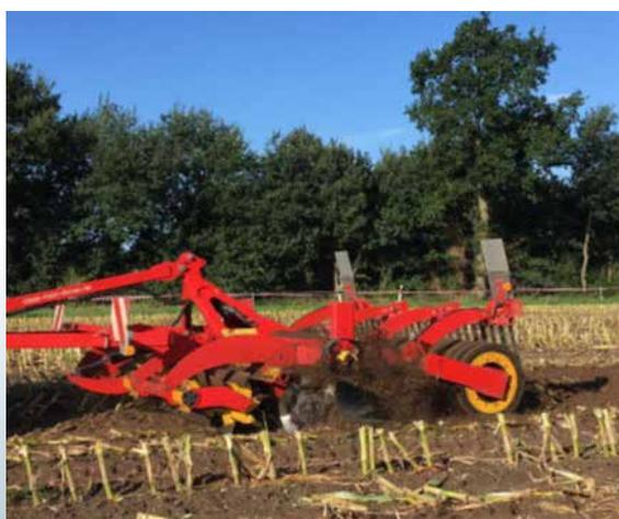
*Carrier disc harrow with CrossCutter Disc in operation in a maize field*
