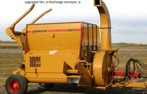
patented chain table in the shredder chamber, a reinforced chain and slat conveyor and a self-loading system.
