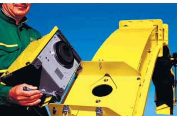
Receiving high-quality feed for cows requires not only feed quality control but also careful nutrients analysis. The best way to monitor the feed quality is to start straight at harvesting. The HarvestLab system from John Deere helps to perform quality control by turning the Self-Propelled Forage Harvester into a fully equipped lab in the field.
