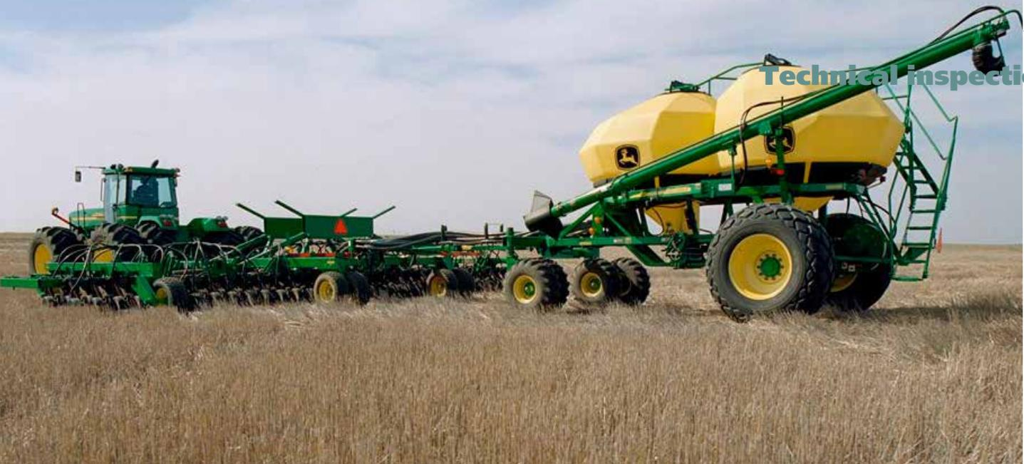
seeding in no-till conditions. This tool is equipped with two rows of openers. The unique one-disc opener allows achieving ideal depth control and seed packing
