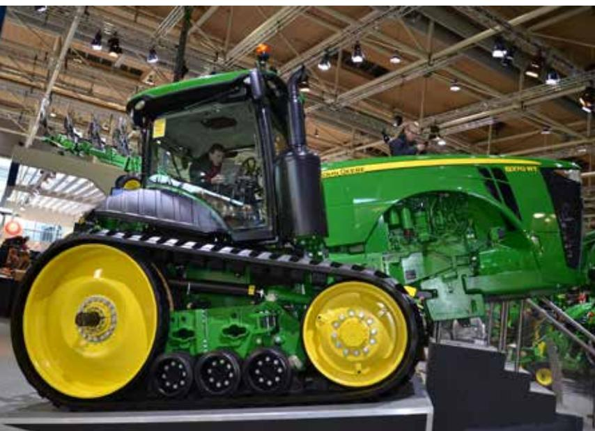
The brand new cab with a 40-degree seat swivel ensures maximum operator comfort. The tracked versions can be fitted with 4,500 to 6,500 mm tracks.
